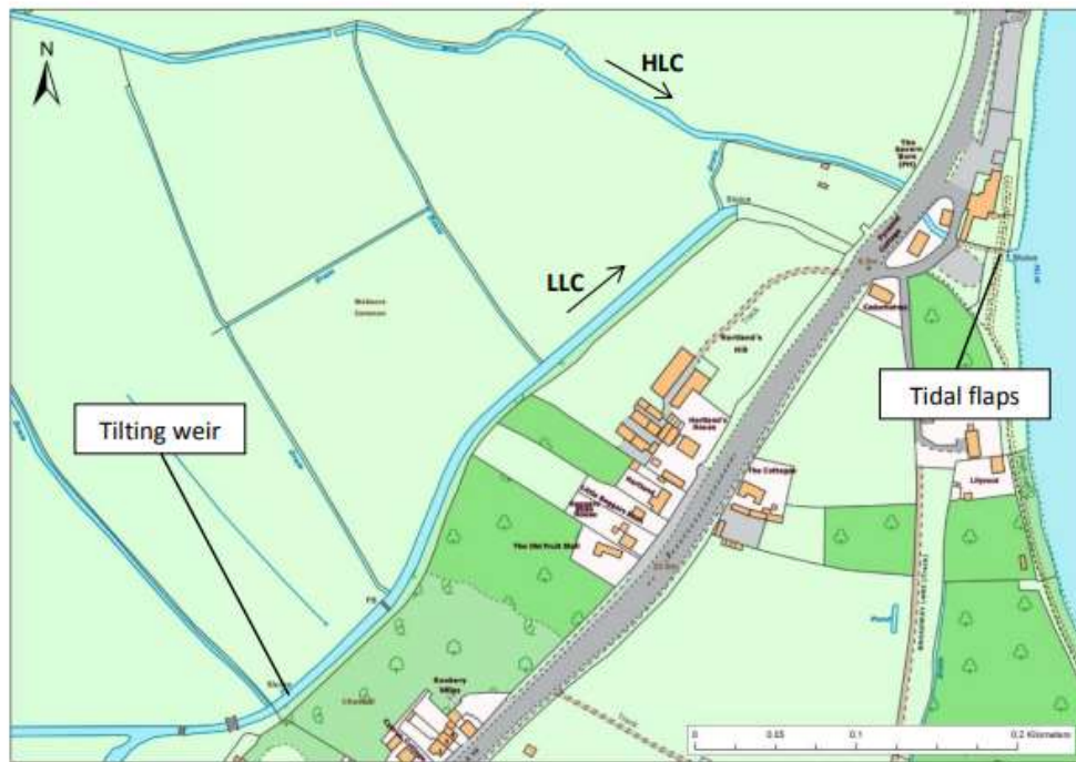
Figure 1.3. Location of the tidal flaps and tilting weir in relation to the High Level Carrier (HLC) and Low Level Carrier (LLC).
